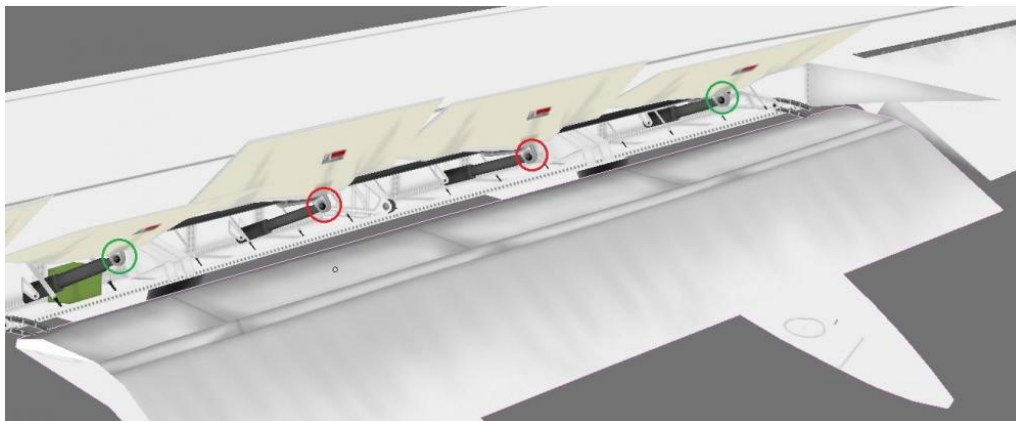
Figure 23: Spoiler actuators example, from [55]
