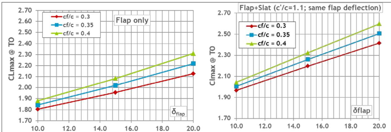
Figure 9: NO SLATS vs. 10% of SLATS chord deflected at the same trailing edge flap angle
