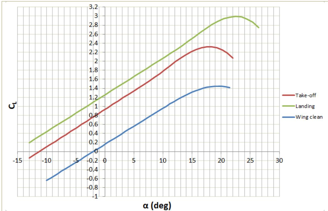
Figure 13: Wing lift curves comparison
