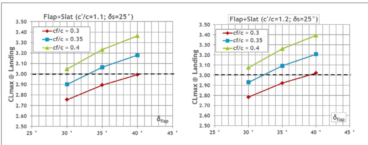
Figure 10: Landing Flap Analysis: 10% vs. 20% of SLATS chord deflected at 25 degrees
