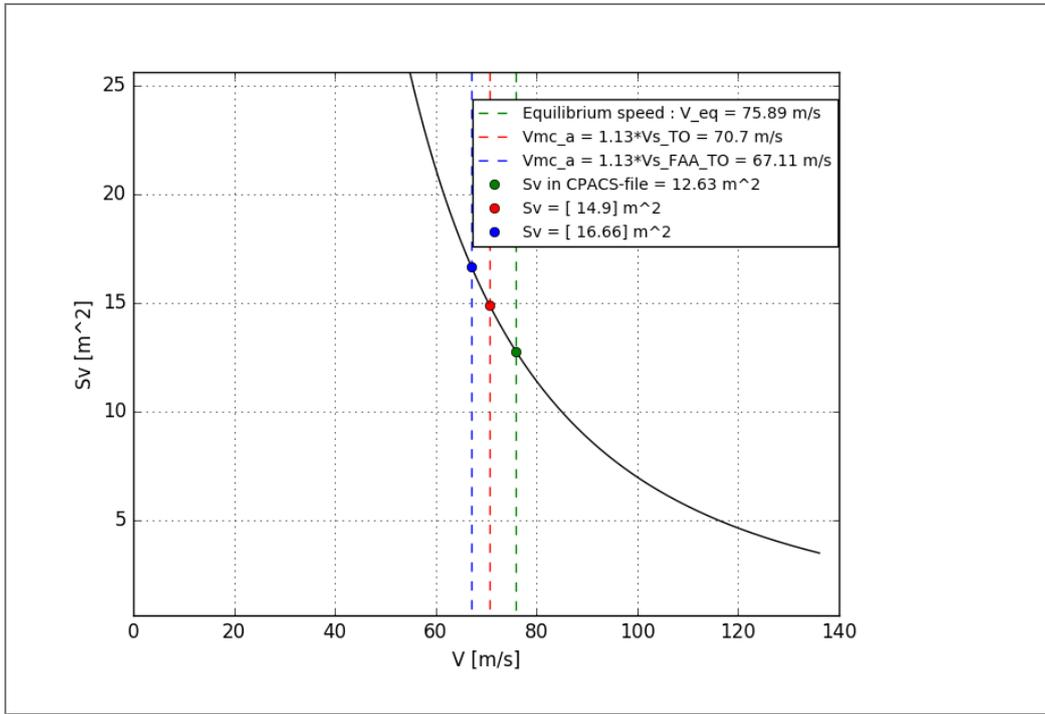
Figure 12: Necessary vertical tail area vs. speed, for equilibrium condition with one engine operative
